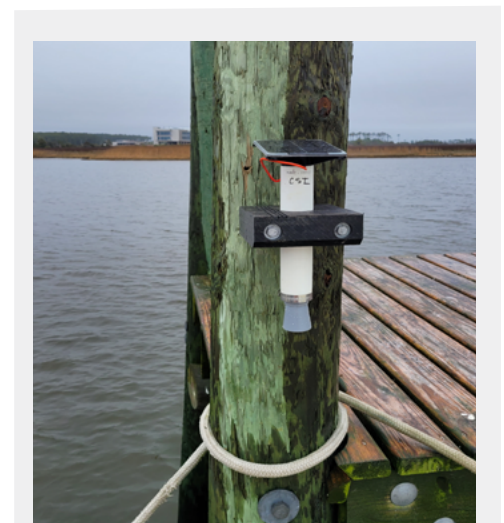
Water level sensors sit above the water and measure the distance from the water to the sensor. The height of the water is collected and relayed in real-time for access on your phone, at home, or in the office.
