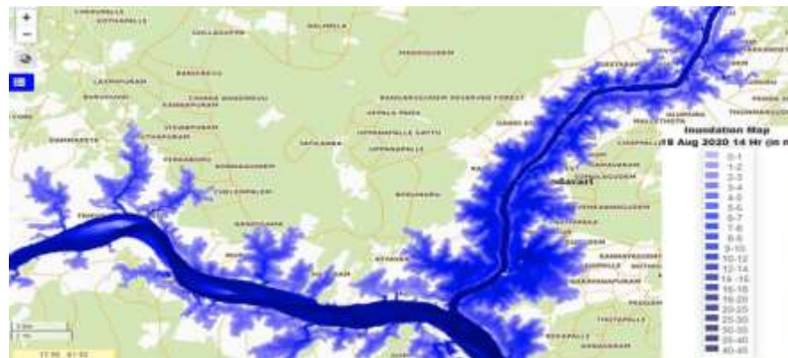
Simulated flood inundation during 2020 flood at Sabari confluence
