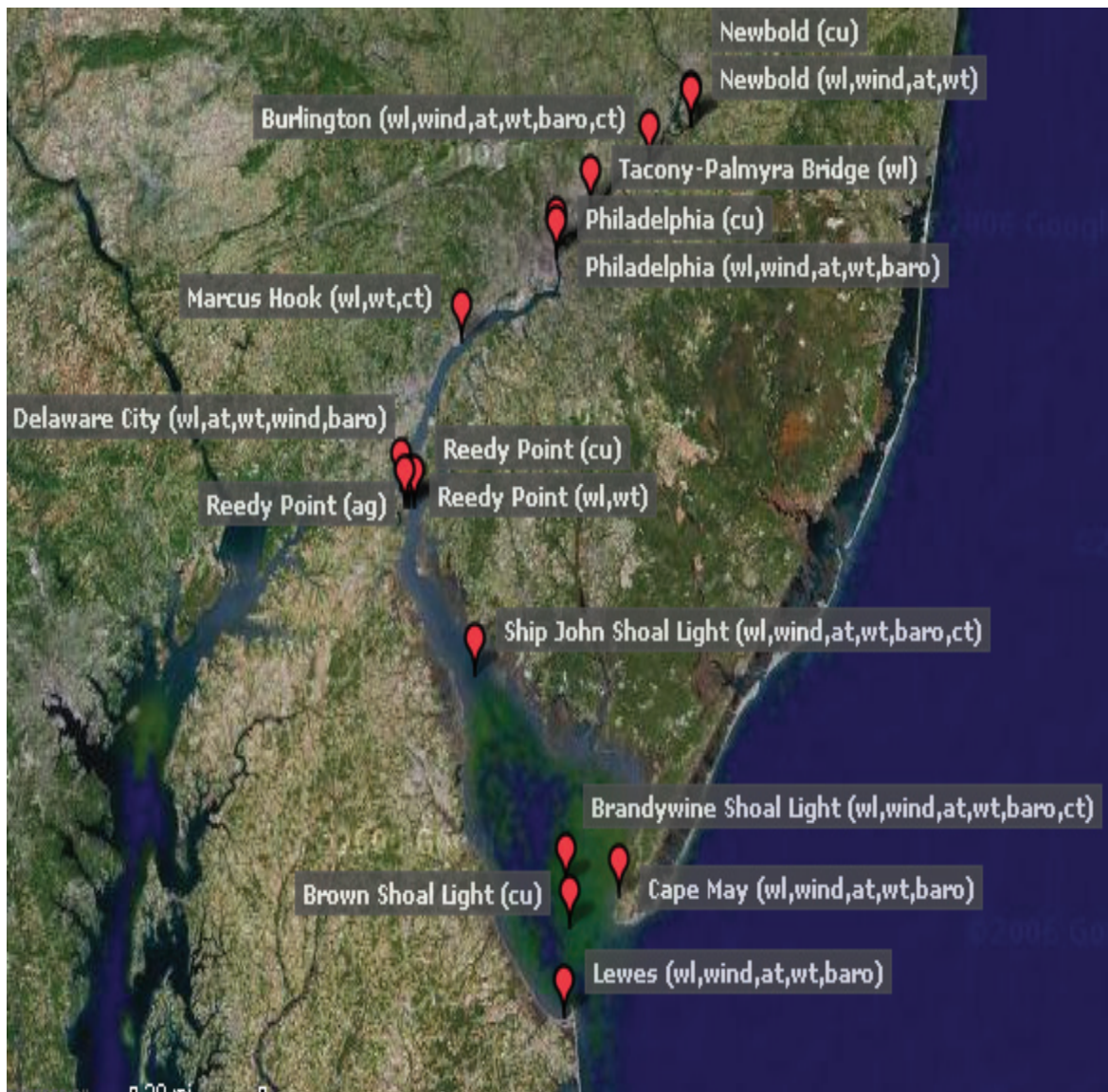
Figure 1.1. Delaware River and Bay PORTS. Note cu=current meter, wl=water level, wind=wind, at=air temperature, wt=water temperature, baro=barometric pressure, and ag=air gap.
