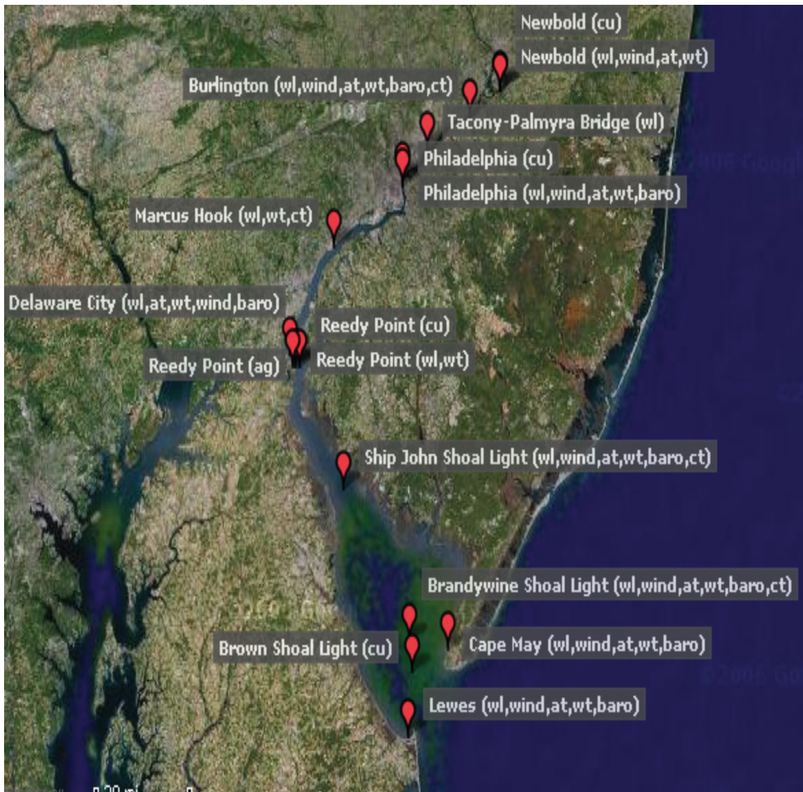
Figure 1. The NOAA/NOS/CO-OPS Delaware River and Bay PORTS. Note cu=current meter, wl=water level, wind=wind, at=air temperature, wt=water temperature, baro=barometric pressure, and ag=air gap. (From http://tidesandcurrents.noaa.gov/ports/index.shtm?port=db )
