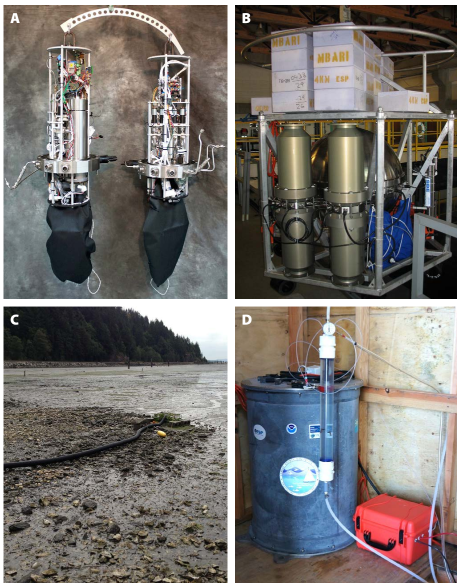
FIGURE 4. External sampling modules for the present-day ESP. (A,B) A deep water sampling module (DWSM) is used to collect water between 50 m and 4,000 m depth, and depressurize it to 1 atm before introduction into the ESP. The DWSM components (A) are located in their own set of cylindrical pressure housings (B) and allow the ESP as shown configured to operate in the deep sea (Ussler et al., 2013; Olins et al., 2017). (C,D) For above-surface applications, a tube is often run to the sample collection site, such as shown here at a shellfish farm at low tide (C). Water is pumped to an accumulator (D), which raises the water pressure slightly to aid in filtering through the ESP (Yamahara et al., 2015; Herfort et al., 2016).
