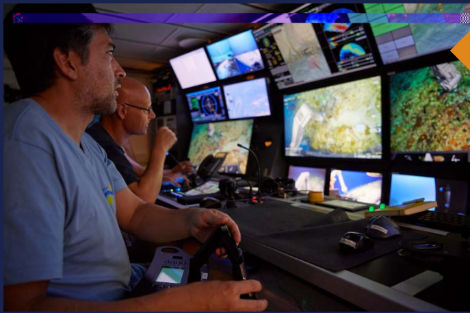
ROV pilots holding position and operating the hydraulic arms to gather samples of ancient, drowned corals. Image credit: SOI
