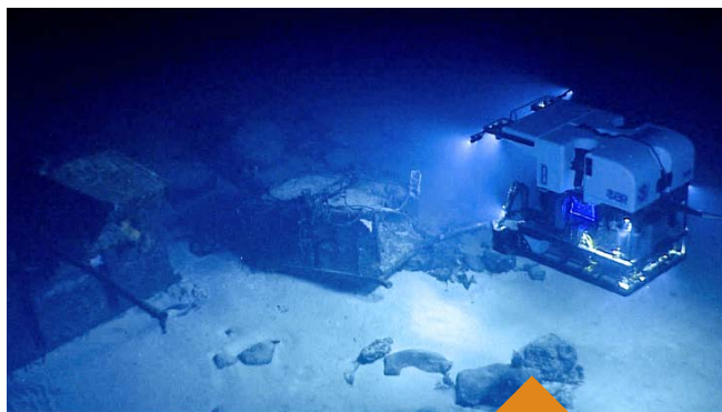
Figure 2. At 785 m depth, ROV Deep Discoverer encountered a World War II-period “rhino barge,” a floating pontoon section that allowed easy access to beaches for offloading of vehicles and supplies following initial amphibious assault landings in the Pacific.
