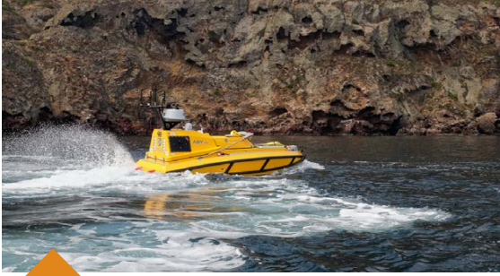
Figure 3. An autonomous surface vehicle (ASV) mapped the shallow submerged shorelines adjacent to the islands.
