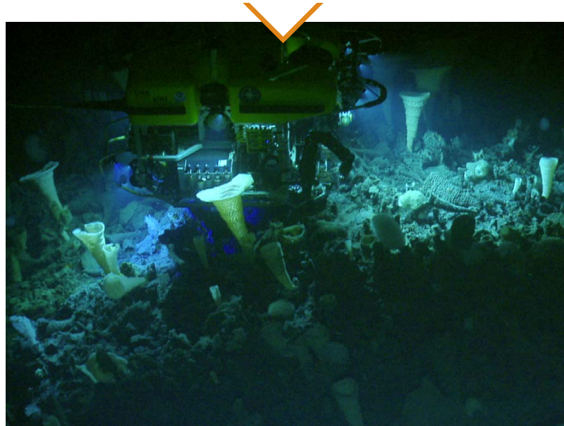
Figure 4. ROV Hercules sampling sponges on top of Explorer Seamount at 800 m depth. Image credit: OET, Northeast Pacific Seamount Expedition Partners
