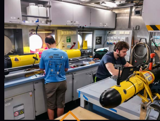
Researchers work on programming and optimizing autonomous vehicles in Falkor 's wet lab. The vehicles pictured are an Iver AUV and a Slocum Glider.
