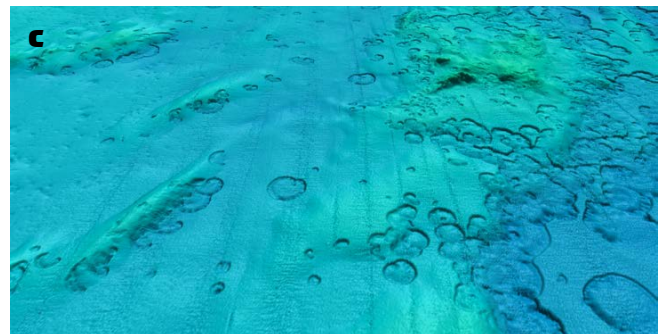
FIGURE 3. (a) Combined, processed bathymetry of the lakebed. (b) ASV BEN bathymetry (6x vertical exaggeration). (c) R/V Storm data used to characterize lakebed and habitats and plan future explorations (6x vertical exaggeration).
