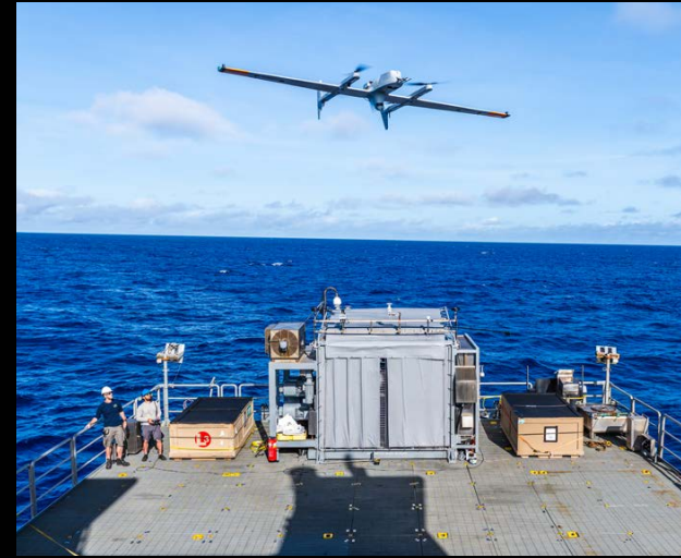
Capable of flying for 12 hours, this L3 Harris HQ-90UAV unmanned aerial vehicle transitions into horizontal flight and vanishes into the distance after a graceful vertical launch.
