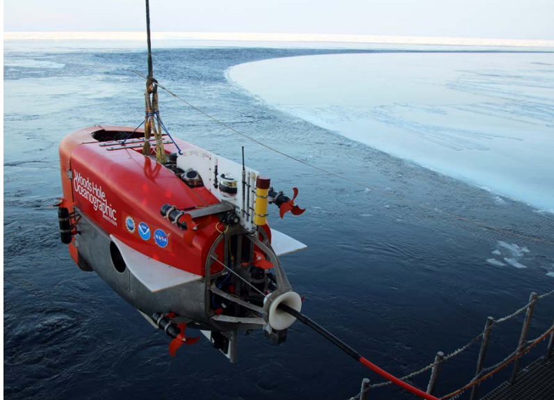
FIGURE 1. The WHOI-developed Nereid Under Ice (NUI) hybrid autonomous vehicle is ready to dive into the Arctic Ocean during the Hot Vents in an Ice-Covered Ocean (HACON) expedition. Image credit: Stefan Buenz, Norges Artiske Universitet
