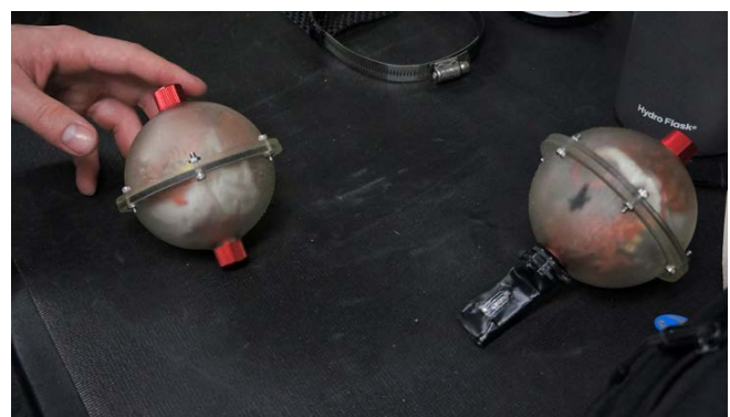
FIGURE 2. These pressure chambers were printed at sea by the URI team using a 3D printer. The chambers were sent to 200 m depth and successfully recovered without any leaks or structure failures.
