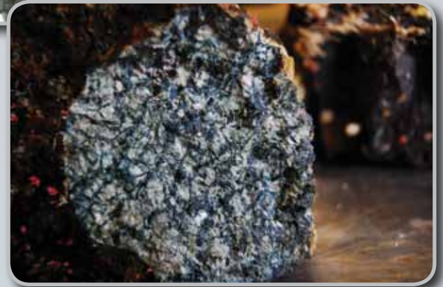
Figure 4. A sample of gabbro, an intrusive rock, that has been altered by hydrothermal fluids.
