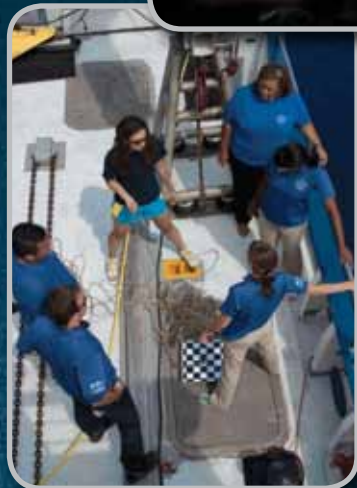
Figure 1. Argonauts deploy an ad hoc Secchi disc to measure the visibility of the water in the Mediterranean Sea. Credit: P. Haydock
