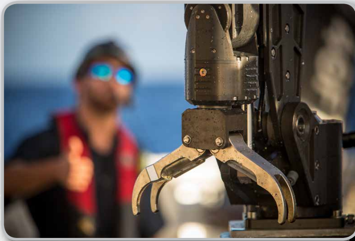
Figure 2. Coral cutter grippers installed on D2's Kraft Telerobotics Predator II manipulator, offshore of Hawaii. Photo by Art Howard/ Courtesy NOAA OER
