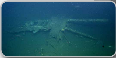
Figure 4. Collapse of the aft spar of Sparrowhawk biplane No. 4's starboard wing is evident in this image.
