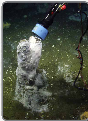
Figure 3. A novel instrument measures eH over one of the chimney-like constructions observed at the Point Dume site.
