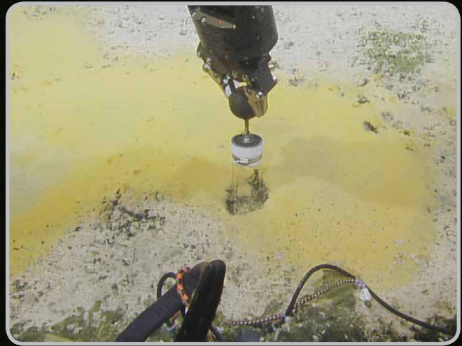
Figure 2. Hercules collects a push core of a bacterial mat and underlying sediment on the Point Dume seeps, offshore Malibu, California.
