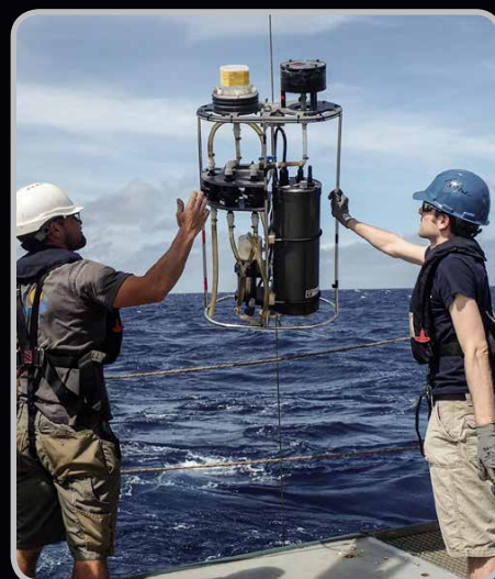
Falkor Bosun Michael Utley and scientist Tristen Horner deploy a McLane Pump off the aft deck to collect seawater in low oxygen zones of the ocean. Photo credit: SOI/Monika Naranjo Gonazles
