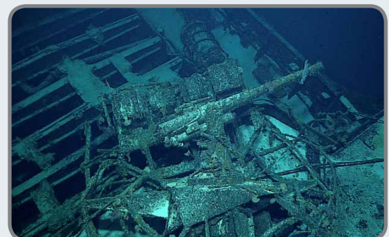
Figure 3. For defensive purposes, Amakasu Maru mounted an 8 cm naval gun on the bow and stern. The gun mounted on the bow has collapsed against the ammunition boxes that are now lined up along the top of the barrel.
