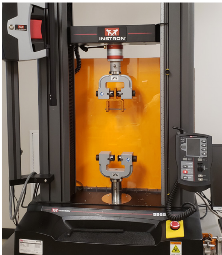
The Instron 5567 electromechanical testing machine has enabled faculty and graduate students to enhance their research. Data has been used in publications as well as preliminary data in support of multiple extramural grant submissions.
