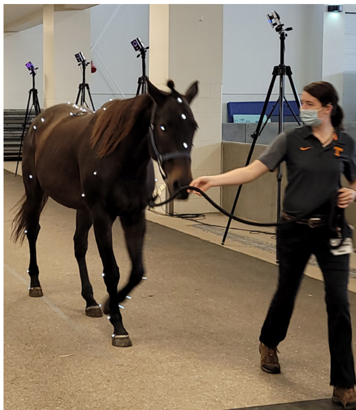
The high-speed cameras of the Vicon motion capture system track markers placed on the animal, allowing researchers to perform complex gait analysis.
