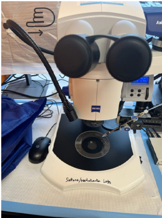
The microinjection system performs microinjections into the tick body, tick anal pore, Drosophila embryos, adult flies, mosquitoes and in vitro grown tick/mosquito cells.
