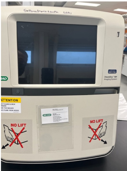
The ChemiDoc MP Imaging System is a full-feature instrument for imaging and analyzing gels and western blots. It is designed to address multiplex fluorescent western blotting, chemiluminescence detection, general gel documentation applications, and stain-free technology imaging needs.
