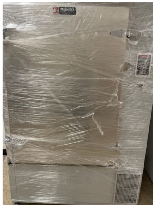
The environmental chamber is an enclosure used to test the effects of specified environmental conditions on biological items, industrial products, materials, and electronic devices and components
