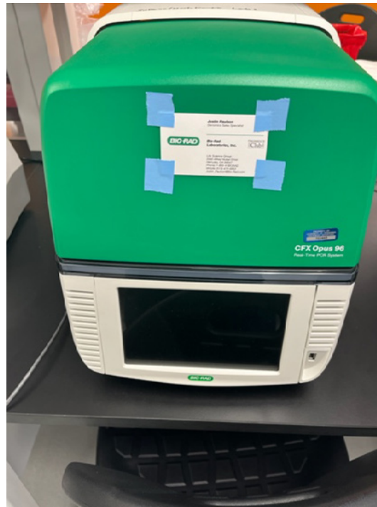
The CFX Opus 96 is a PCR system. A PCR system is used to make millions of copies of an initially small segment of DNA. This allows scientists to amplify DNA enough to study in detail, making it an incredibly valuable piece of equipment in both clinical and research settings.
