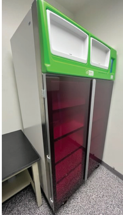
This Aria Bio-C36 ventilated cabinet allows for biosafety so that laboratory work can be performed safely by personnel.
