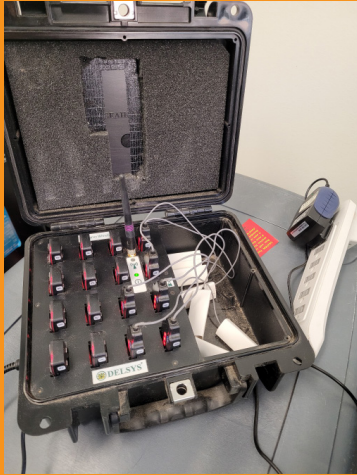
The Delsys-Trigno Avanti Digital Base Station is an inertial motion unit combined with an EMG (electromyography) system that synchronizes with the Vicon motion capture system for complete biomechanical analysis. This device is used in the Equine Performance and Rehabilitation Center to study movement in equine athletes to advance the science of locomotion disorders.
