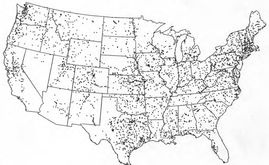
Figure 1. Locations of U.S. Geological Survey stream-gaging stations that are used by the National Weather Service to develop river forecasts.
