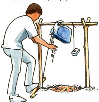
Attach one end of string to water container lid and the other end to the foot lever stick. Adjust the lengh so container tips when foot stick is pressed.
