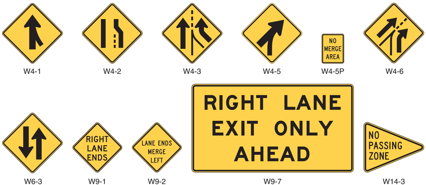
Figure 2C-8. Merging and Passing Signs and Plaques
