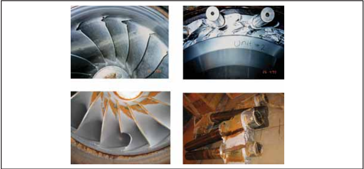
Figure 29: Sediment Induced wear of Hydro-turbine (Bishwakarma MB. 2008)
