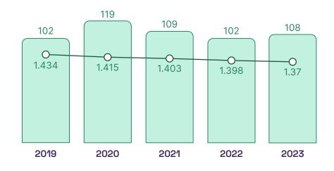
The increase in power consumption in 2020 is attributed to the expansion of our server deployment that year. Optimizations related to UPS (Uninterruptible Power Supplies) and temperature adjustments in IT rooms have facilitated a reduction in power consumption in 2021.
