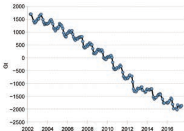
FIG. 5.12. Change in the total mass (Gt) of the Greenland ice sheet between Apr 2002 and Jun 2017, estimated from GRACE measurements. (Due to the decommissioning of the GRACE satellite, no data are available after Jun 2017.) Data are based on an unweighted average of JPL RL05, GFZ RL05, and CSR RL05 solutions, which reduce noise in the GRACE data for 2017 (Sasgen et al. 2012).
