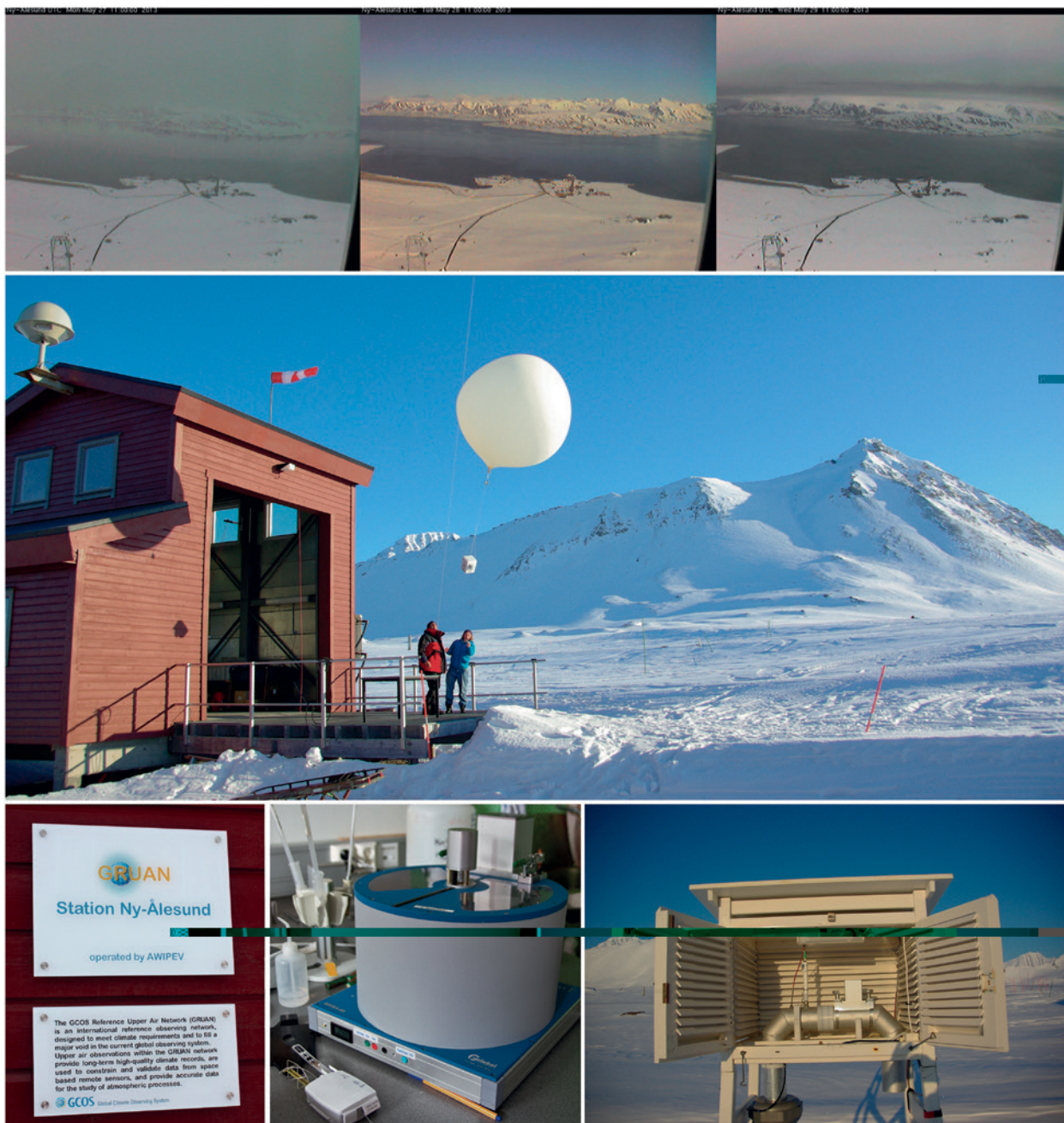
FIG. 5. Images of GRUAN operations at Ny-Ålesund. (top) Sequence of launch condition photos from the Norwegian Polar Institute webcam on Zeppelin Mountain on 27–29 May 2013. (middle) Launch of an ozonesonde. (from bottom left to bottom right) GRUAN site plaque, 100% relative humidity chamber, and ventilated weather hut for outside launch condition comparison.
