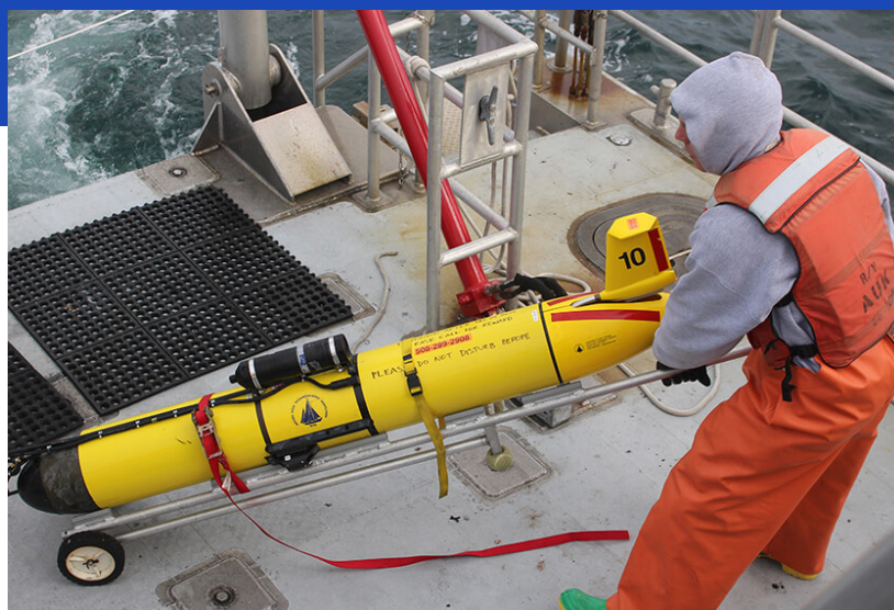
A researcher gets ready to launch a type of autonomous underwater vehicle, called a "glider." The glider records all sounds as it follows a programmed path. Photo: Anne Smrcina/NOAA
