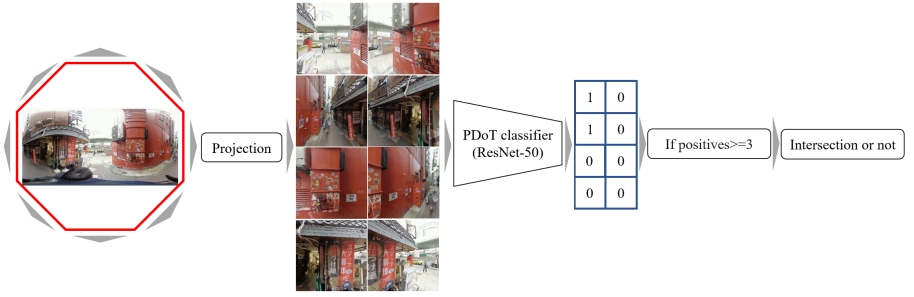
Figure 3: Illustration of the proposed method. Multiple non-overlapping perspective images of the 45^\circ \times 45^\circ FoV are cropped in eight view directions and our PDoT classifier is applied to individual images. If three or more PDoTs are detected, the 360^\circ image is classified as an intersection frame.
