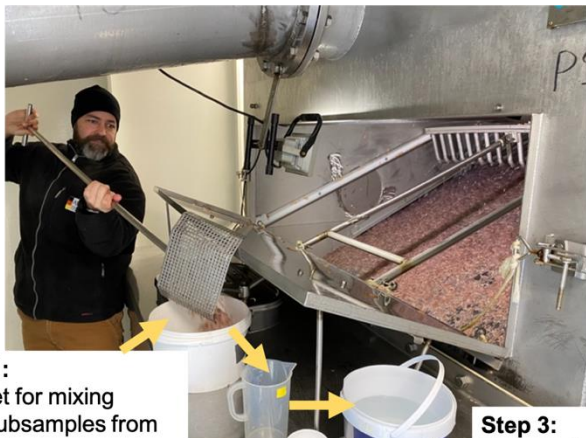
Step 2: Fill two graduated measuring jugs with krill to the ~ 200ml mark and the ~ 50-100ml mark, respectively.
