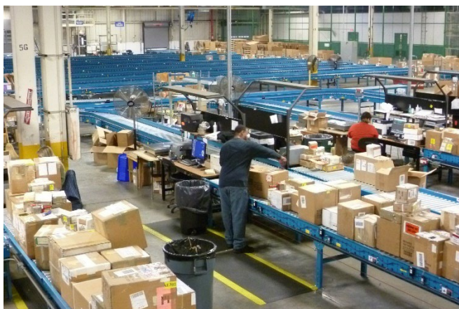
Figure B2. Conveyors and workstations for small parcel line receiving. Photo by NIOSH.
