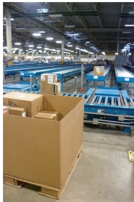
Figure B4. An unused conveyor blocking the pathway between the end of a conveyor line and the triwall container where boxes were placed. Photo by NIOSH.
