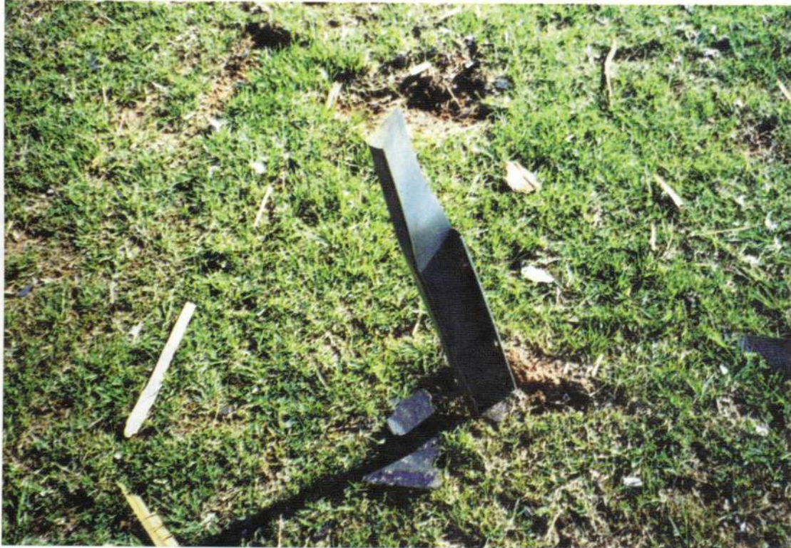
Figure 37. C-Section Steel Projectile
