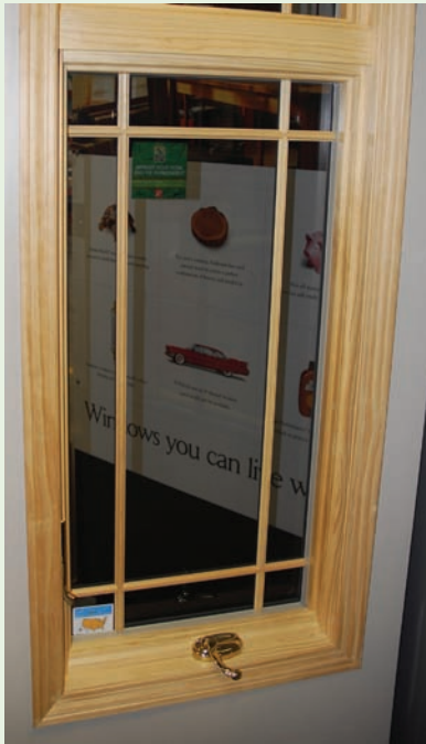
Figure 4-19. This attractive window can be fitted with energy-efficient glass, impact-resistant glass, or both. The impact-resistant glass consists of a laminate or film sandwiched between two glass panes. The frames are reinforced and the hinges have extra fasteners to withstand high-wind events. Wind-generated debris may crack the glass, but the laminate will hold the windowpane together in the frame and prevent breaching of the wind- and rain-resistant envelope. After the storm, the glass will need to be replaced. Image courtesy of Dennis Hwang
