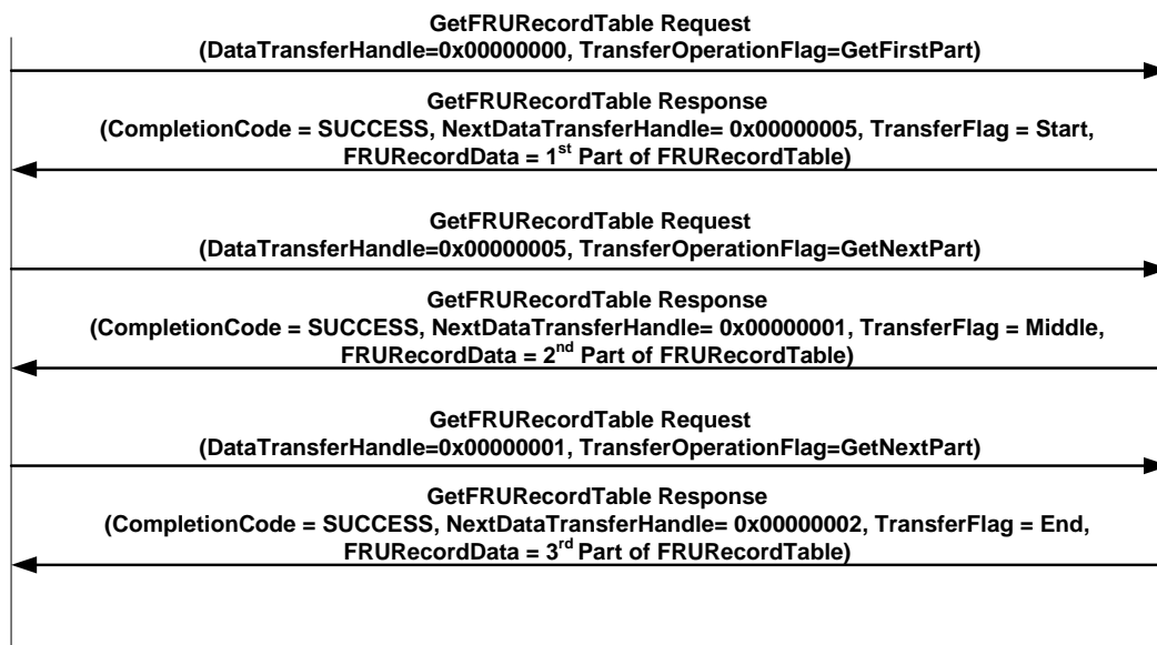
316 Figure 1 – Multipart FRU Record Table transfer using the GetFRURecordTable Command
