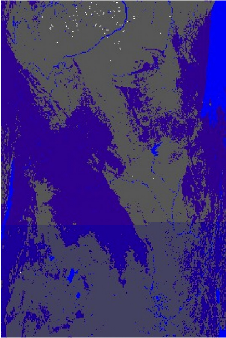
Figure 2: Example MOD14 granule with water shown in blue, clouds in purple, clear land in grey, and active fires in white. The along-track direction points toward the top of the page.
