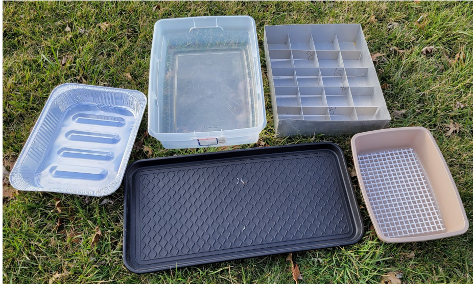
Figure 2. Examples of pans that are acceptable for the simple pan test. Dividers inside the pan to reduce material bouncing will improve results.
