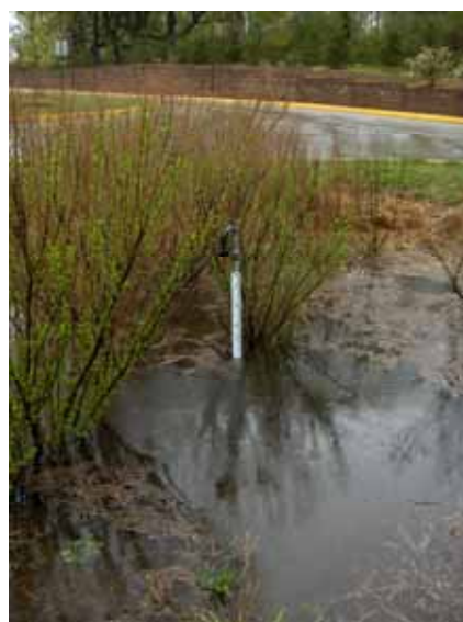
FIGURE 5-51 Staff gauge attached to ultrasonic sensor after a storm. SOURCE: VUSP.
