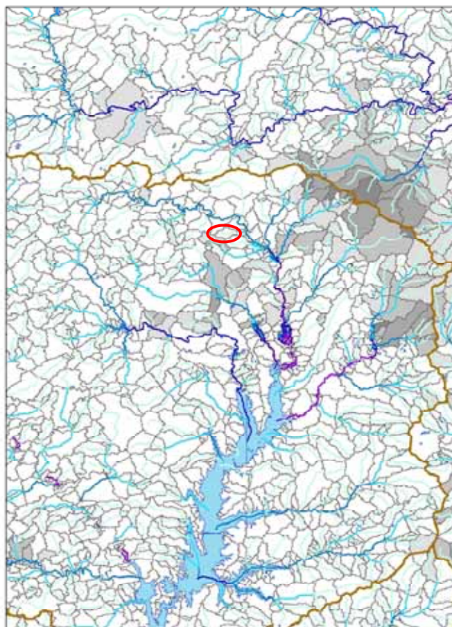
FIGURE 4-14 The drainage area to Jordan Lake, a major drinking water reservoir in the Triangle area of North Carolina, is under nutrient-sensitive rules, requiring reductions in total nitrogen and phosphorus. Drainage flowlines and catchment areas are from NHDplus, and are shaded according to their percentage of industrial and commercial land cover from the NLCD. The area outlined in red is a small urban catchment, detailed in Figure 4-15, and comprised of a wooded central region, surrounded by residential and institutional land use.
