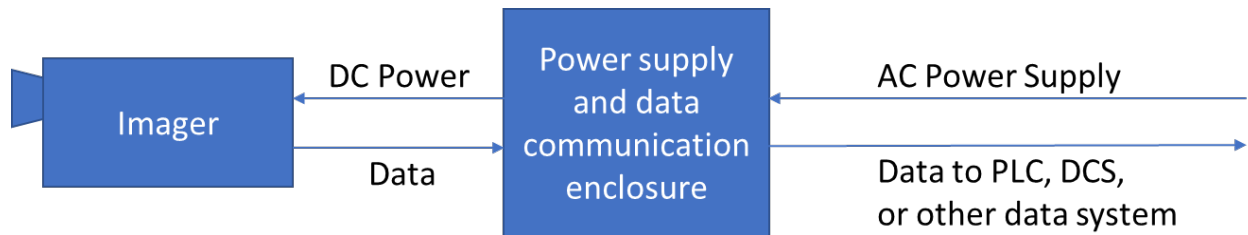
Figure 1. Schematic showing typical equipment for the VISR method
