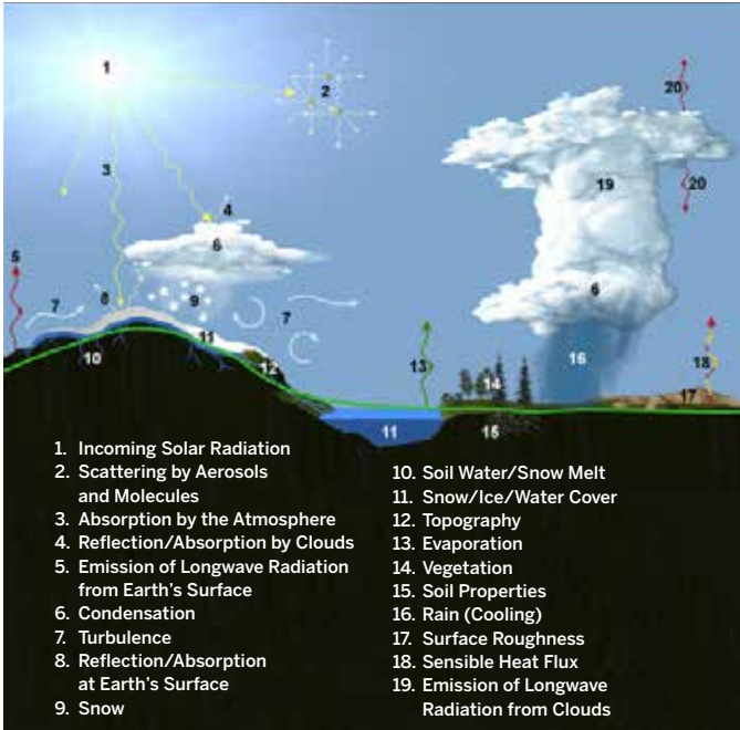
A summary of the various parts of NWP modeling that are parameterized.
