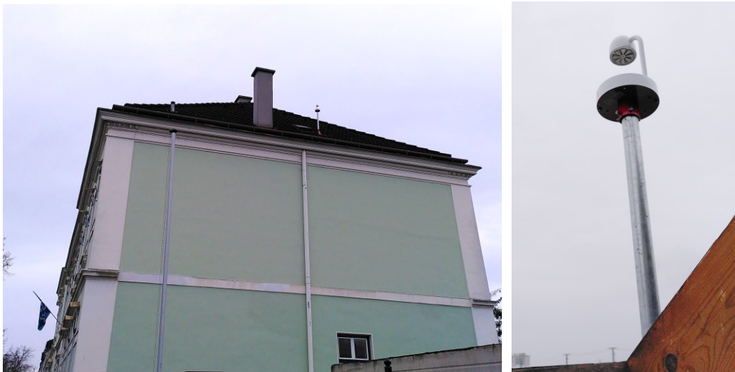
Figure 2-8. Electric Field Mill installed at the ESSL Research and Training Centre in Wiener Neustadt.
