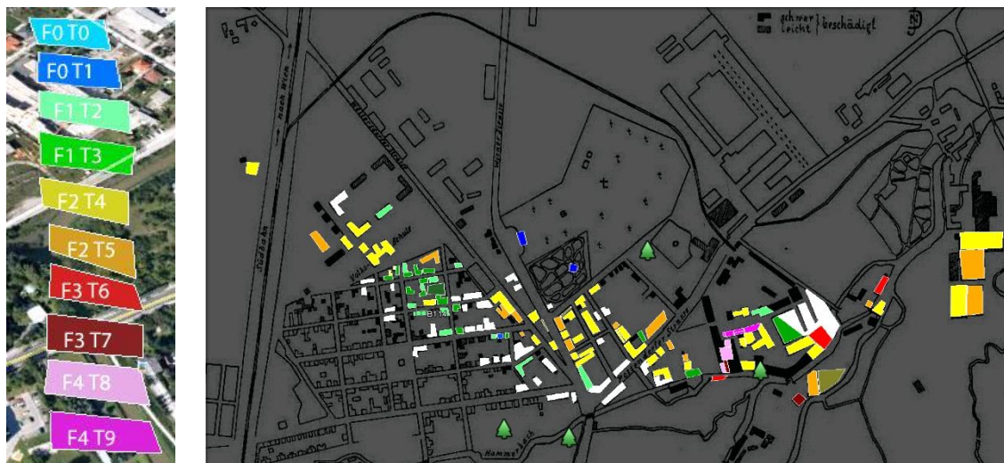
Top: Damage track produced by the tornado on 10 July 1916 across the northern part of Wiener Neustadt.
