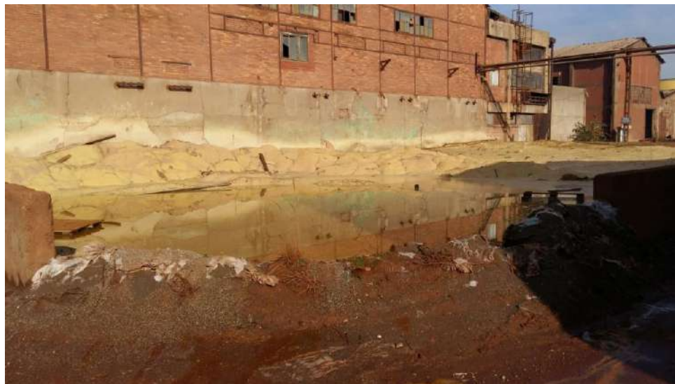
Figure 15. PbAg precipitate in a pond inside Zorka - Obojena Metalurgija in Šabac [Picture by Marco Falconi]
