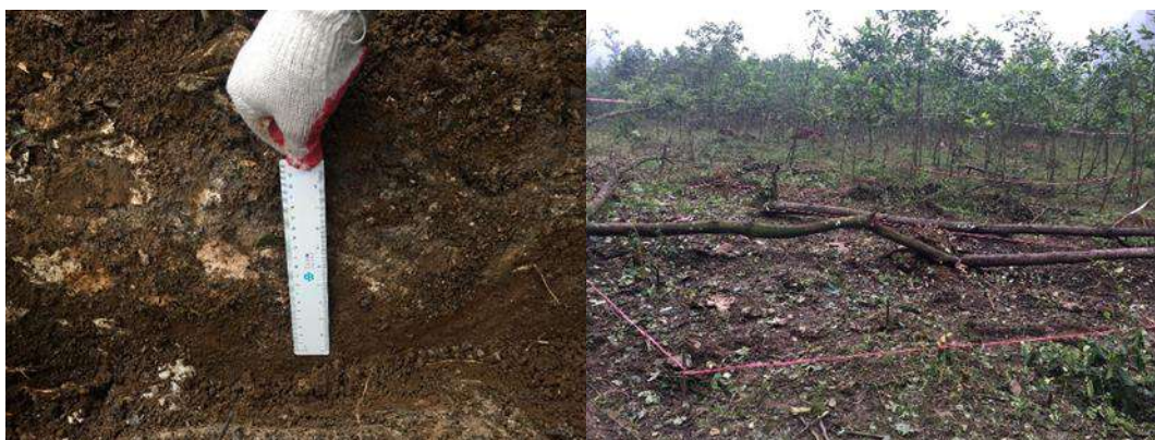
Figure 3. Left: Shallow trench to map the DDT. Right: Hotspot indicated with colored rope (From Tauw, 2015)
