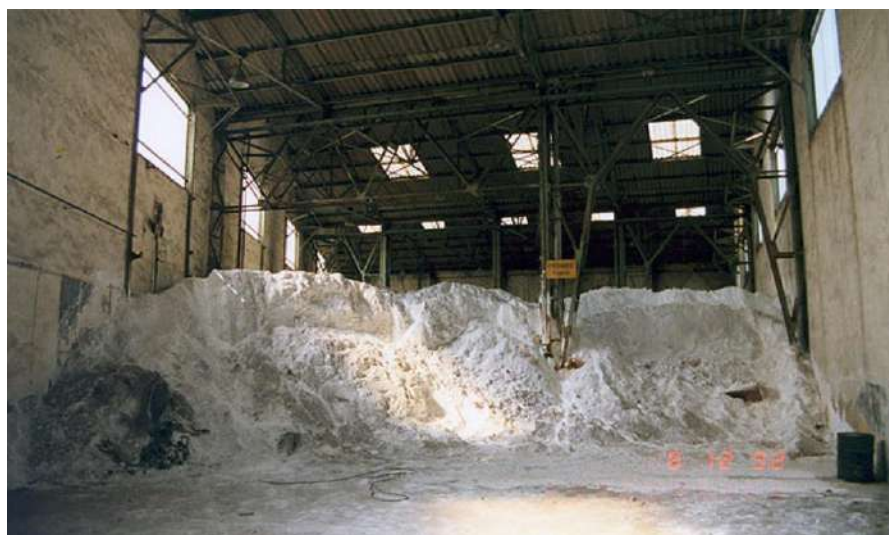
Photo 4. Waste HCH isomers being collected inside a former lindane production facility in Basque Country Region of Spain. (©IHOBE, Basque Country)
