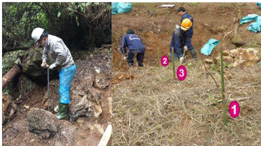
Figure 4. Left: Soil sampling. Right: Transact to map the bomb crater (From Tauw, 2015)
