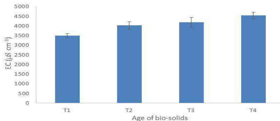
Figure 3. Effect of age of bio-solids (x-axis) on electrolytic conductivity, EC (y-axis) from Bugolobi Wastewater Treatment Plant as of March 27, 2014. T1, T2, T3 and T4 denote: fresh, settling, maturing and mature bio-solids, respectively.
