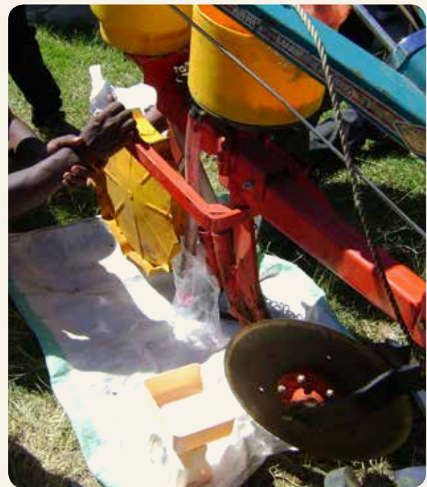
Plate 4.10 Calibration of seed delivery for a 2WT-drawn no-till planter © B. Sims
