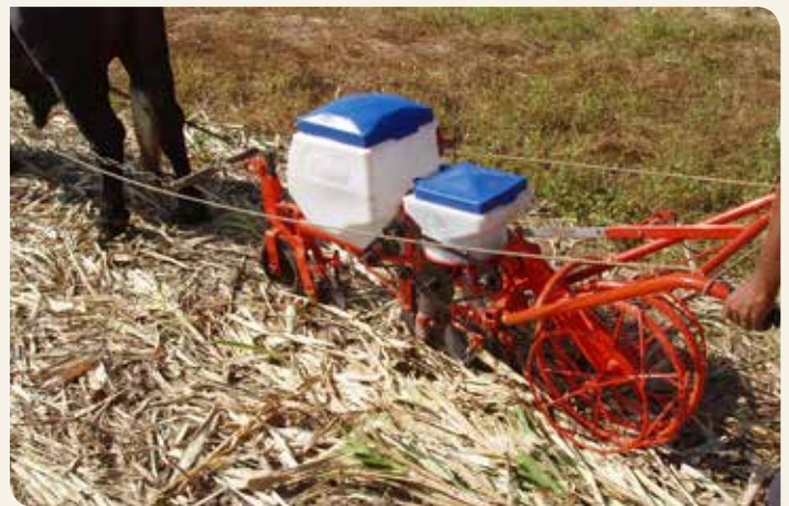
Plate 1.3 Animal-drawn no-till planter with double offset disc openers © B. Sims
