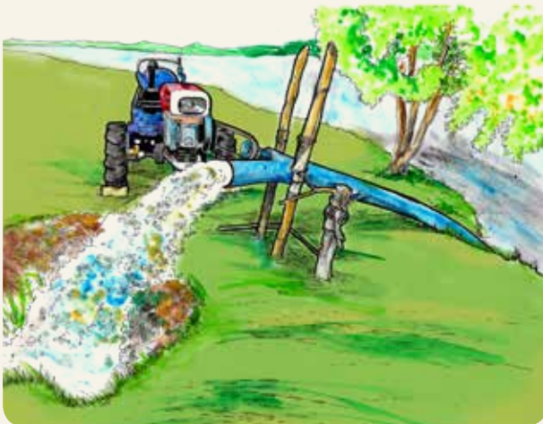
Plate 4.17 Centrifugal pump driven by engine connected directly to power-take-off shaft
