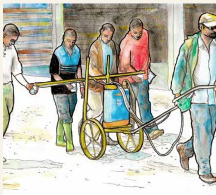
Plate 4.12 Calibration of an operator-pulled four-nozzle sprayer
