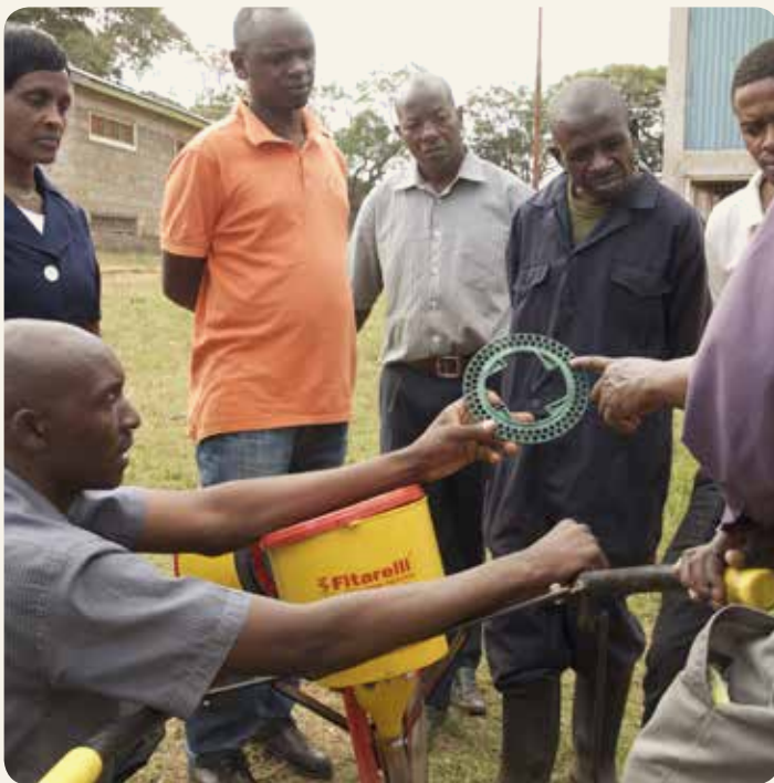
Plate 4.9 Horizontal rotating seed disc (for beans) for an animal-drawn direct seed planter © FAO/IS. SantosValle
