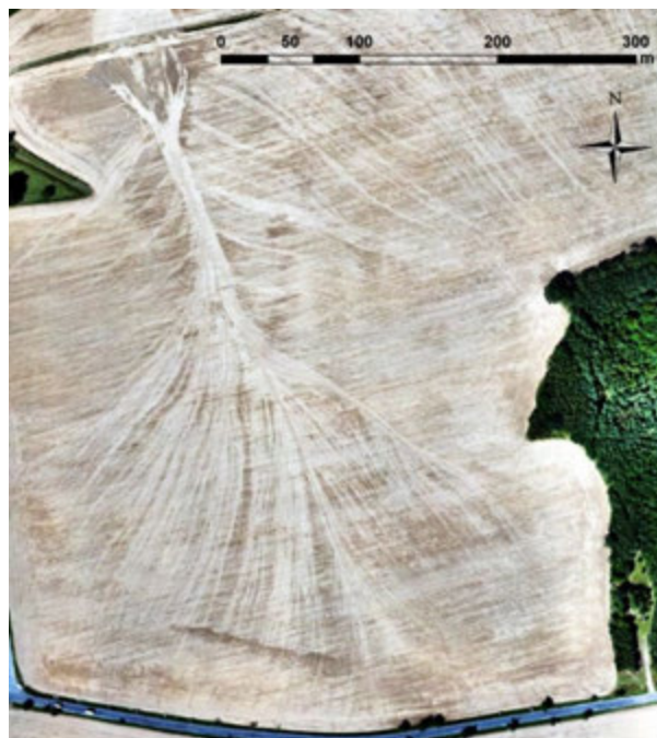
Figure 1: Rill and ephemeral gully pattern in Lbosin field (August 2017)
