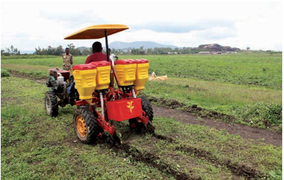
Two-wheel tractor with a direct seeder implement for Conservation Agriculture.
