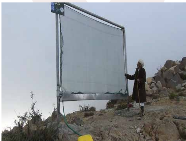
FIGURE 47 Fog harvesting screen in Yemen
