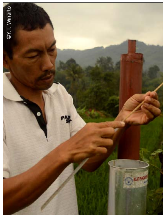
Figure C-2: Farmer uses a ruler to measure the wetted part of a dipstick, indicating how many mm of water had fallen over the last 24 hours
