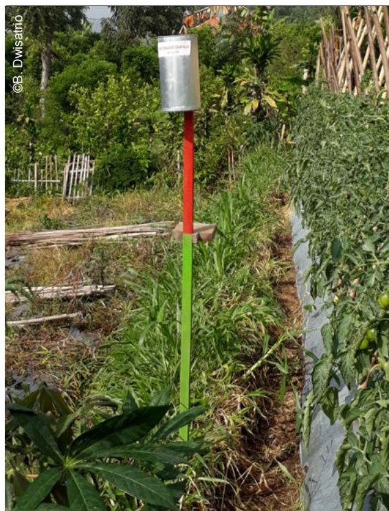
Figure C-1: Indramayu farmer's homemade rain gauge
