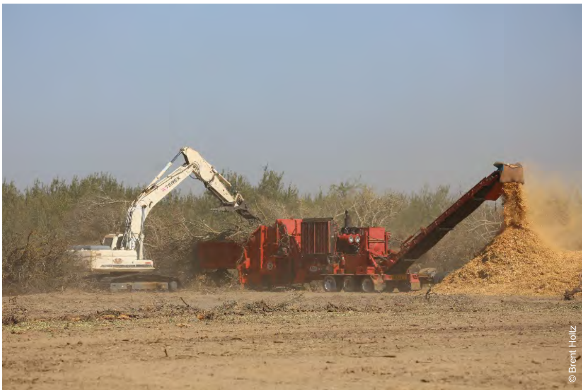
Photo 100. The process of on-site grinding at an orchard in San Joaquin Valley, California, the United States of America
