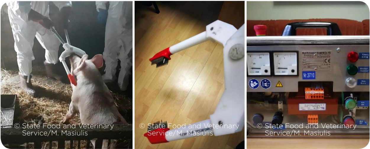
Figure 3. Electrocutation: scissor-type tongs and application of current to the head of the pig spanning the brain
