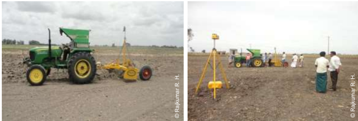
Figure 2. Operation of laser land leveling
