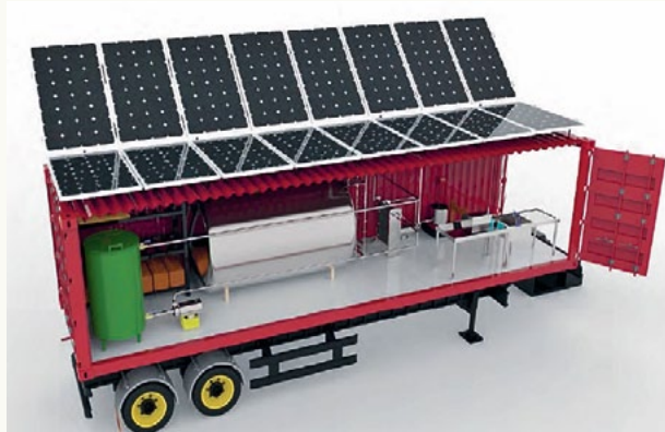
FIGURE 4.19. Mobile milk cooling centre using solar panels and ice bank.
