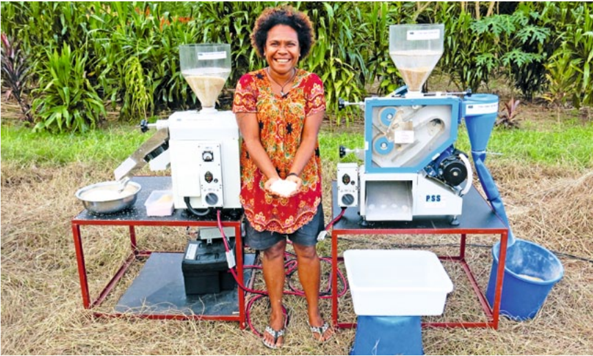
FIGURE 4.48. Solar-powered electric motor driven rice husking mills.
