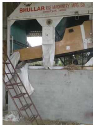
The rice falls from the shaker into bucket elevators, which transport it up into the dryer.
