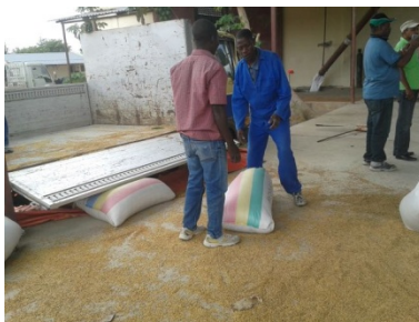
Delivery of paddy in bags from the farmer at the factory. The transport is mostly provided by EOZ. The bags are emptied onto the inclined shaker to remove dust and impurities.
