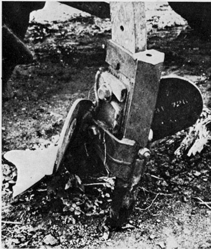
FIGURE 37. - Subsoiling tine integral with lister body. (Photo Ministry of Agriculture Forestry and Wildlife, Tanzania.)
