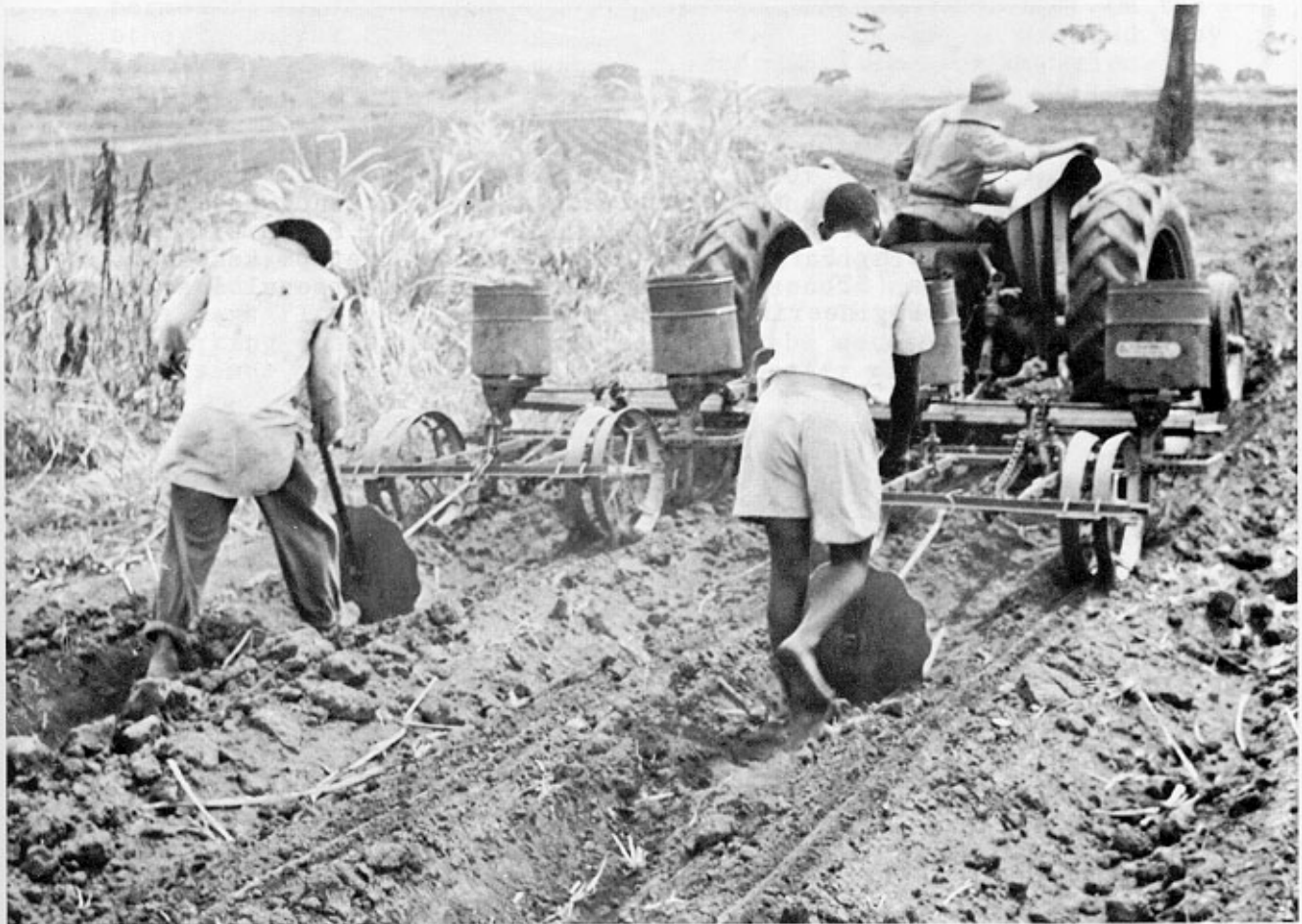
FIGURE 26. - Hand operated ridge tying units at the Cotton Research Station, Namulonge in Uganda (31). (Photo courtesy of National Institute of Agricultural Engineering, U.K.)
