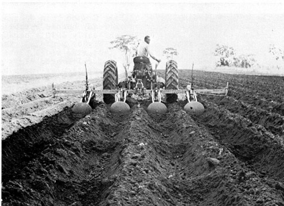
FIGURE 30. - Similar equipment in use on the Cotton Research Station in Uganda splitting and retying ridges made the previous season. (Photo courtesy of National Institute of Agricultural Engineering, U.K.)
