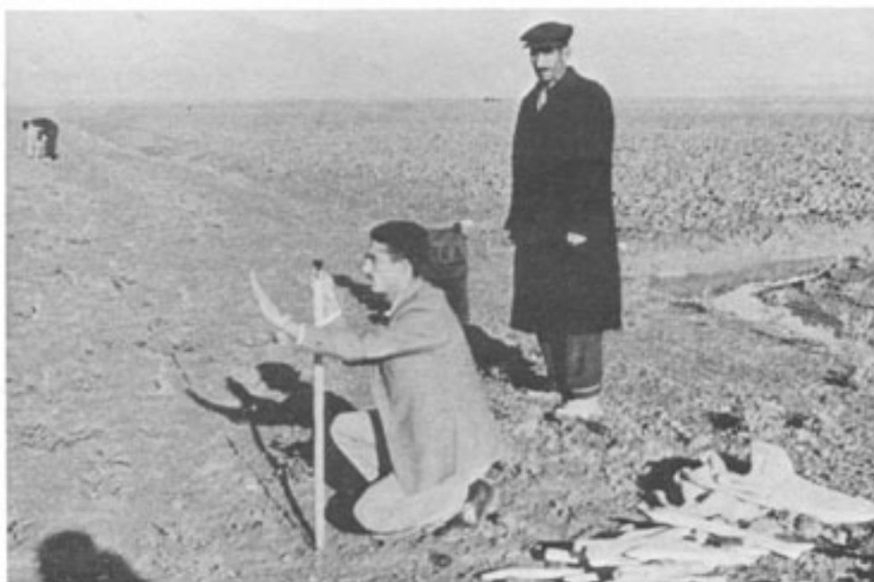
Picture 1. The team leader fixed the "left point" and adjusts the trial's right angle. (Refer to Section 2.5.1.)
