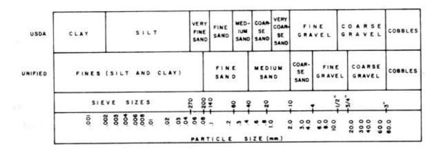
Figure 1. Comparison of particle sizes of soils in the USDA pedological and the unified engineering soil classification systems (adapted from PCA, 1962).
