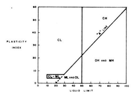
Figure 2. Groupings of soils in the unified soil classification system in the fine grained sizes, showing relationships between the categories and the liquid limit and plasticity index (adapted from PCA, 1962). See Table 2 for an explanation of the symbols.
